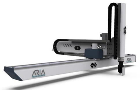
The three-axis linear robot has Cartesian axes which are operated via the robot controller. Our different robotic solutions cater to the digitalization of the manufacturing process, providing our customers with the ability to increase productivity, Lower manufacturing costs, enhance flexibility and repurposing, Improve precision and accuracy, ensure highest quality standards and consistency, and increase work safety.
